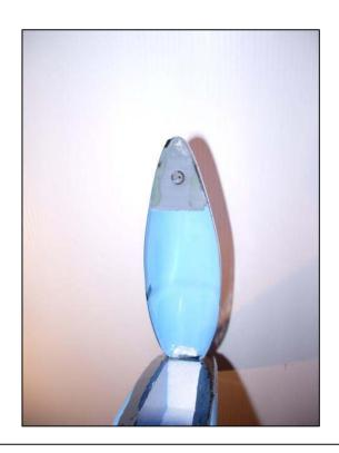
Drill a small hole and glue magnet to the Coroplast at the rear of the canopy.
