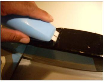
Test fit the hinge. Then glue into place.
