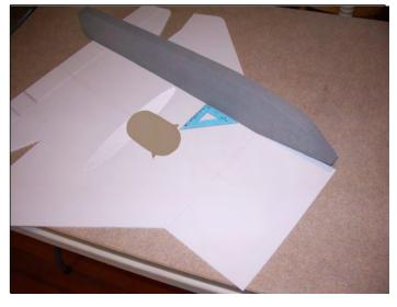
Ensure the nacelle is parallel and 90 degrees to prop slot in wing. You have some time to make slight adjustments before epoxy cures but move quickly.
