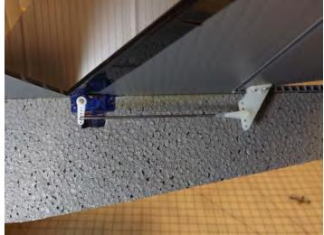
Connect the push rod to the servo arm 2<sup>nd</sup> hole from end and control horn middle hole.
