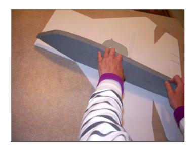
Be sure that the nacelle is properly aligned with crease
