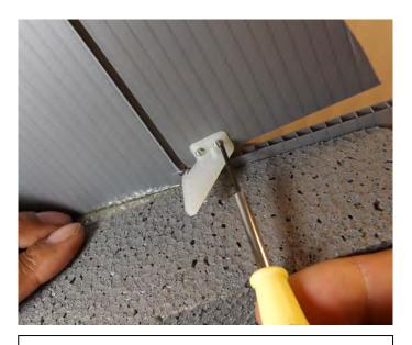
Attach the control horn to the right elevon, don't over tighten.
