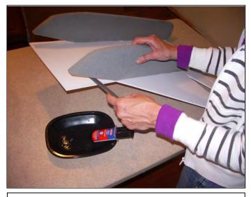
Now apply 5-minute epoxy to the slanted sections on both nacelles.
