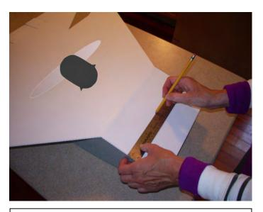
Turn the wing over, measure and mark on the top the center of the wing
