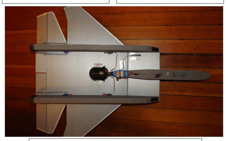
Use servo Y leads to route wires as shown in photo. Once wires are neatly placed they can be taped in place in the slots and to bottom of wing with clear packaging tape or vinyl tape to match the color of the wing. Care must be taken that the wires and receiver antenna do not become entangle or severed by the fan blades
