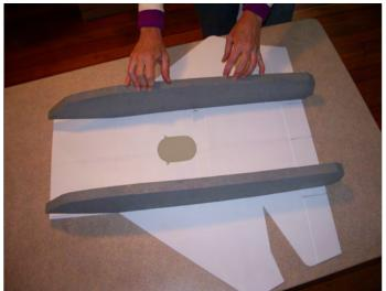
Repeat the steps to attach the second nacelle to the wing. Nacelles should be straight and parallel
