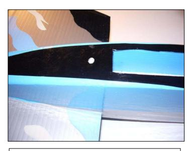
Drill a hole the same size as the magnet near the battery box, position it such that it will align with the magnet on the canopy. Ensure the polarity of the magnet is such that they are attracted when the canopy is closed. Epoxy the magnet in place
