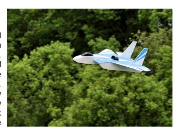
The T-15 is very rugged and can take a lot of abuse however in extreme heat, the plastic can warp. Avoid leaving it in a hot car or storing it in a manner that distorts the wing or tail. Also in extreme cold this plastic may become stiff and brittle and lose some of its impact resistance.
