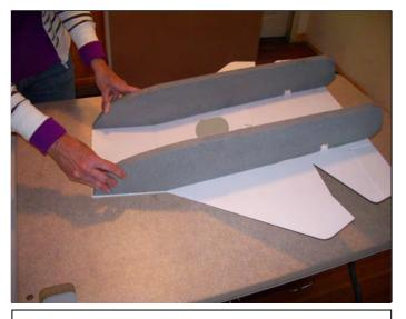
Press both nacelles to leading edge of the wing applying pressure on a smooth flat surface for 5 minutes until the epoxy cures
