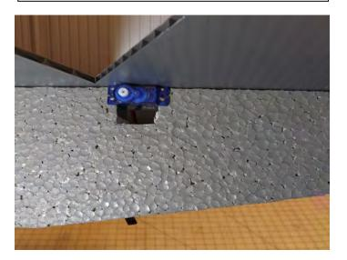
Install the outboard servo into the mounting hole and glue in place, stacked on top of inboard servo. We recommend 9 gram sub micro or similar type servo.
