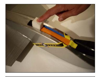
The foam filler block that is included uses the rest of the space and locks the battery in place. Place it behind the battery for flying in wind. You also may want to use this placement for the first few flights to get used to the plane.
