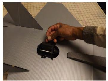
Bolt motor to mount with 3mm x 14mm bolts included.
