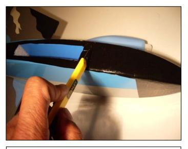
Cut a slit 1/4 " in front of the battery box for the canopy hinge.
