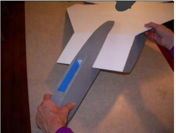
Apply 5 minute epoxy to both side of fuselage wing slot. Slide the fuselage onto the wing. Be sure that the fuselage is centered straight and square to wing.
