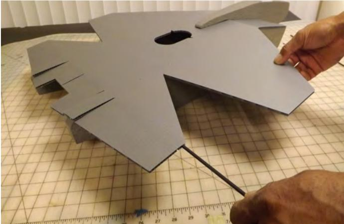
Apply a little 5 minute epoxy to the 24 inch carbon fiber shaft then insert it in a tail approximately 1st flute from leading edge (see photo)
