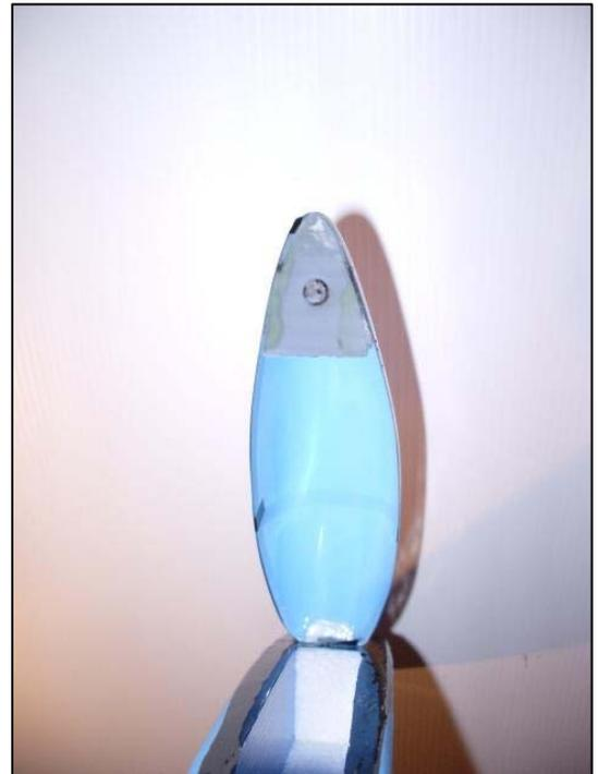
Drill a small hole and glue magnet to the Coroplast at the rear of the canopy.
