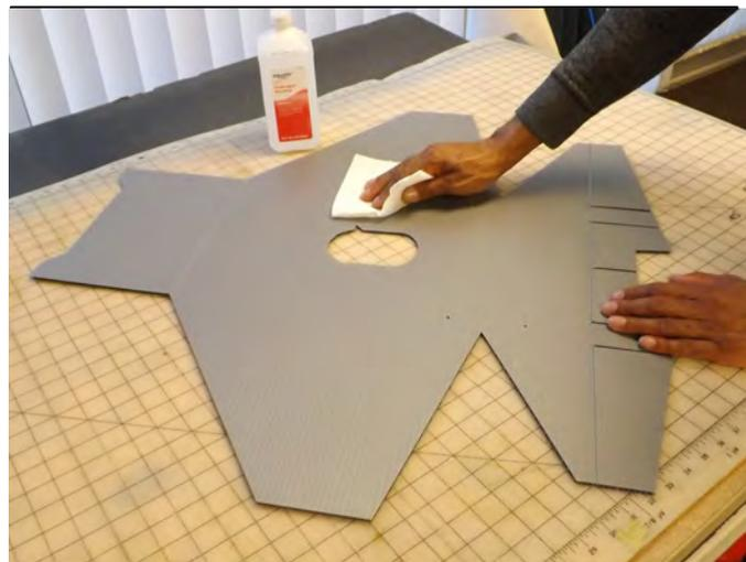
Clean the bottom of the wing with rubbing alcohol before gluing
