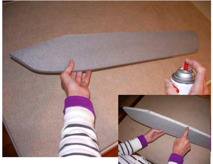
It is recommended to apply the covering material or paint prior to assembling the model. Do **NOT** apply covering to the top edge and slant of the nacelle (**see insert**)
