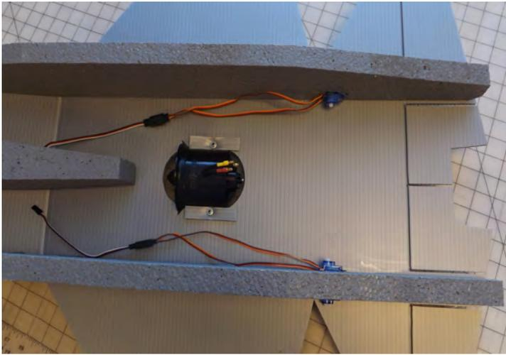
Servo wire exits on inside of nacelle.
