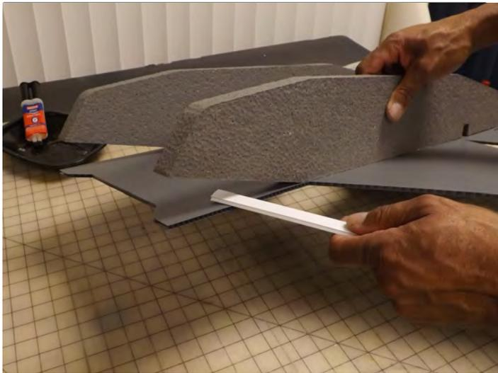
Now apply 5-minute epoxy to the slanted sections on both nacelles.
