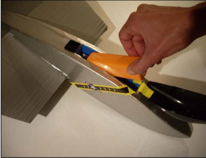
The battery box located on the front of the plane is designed to accept 4-cell lipo 14.8 volt 2200 mah or 2600 mah battery.
