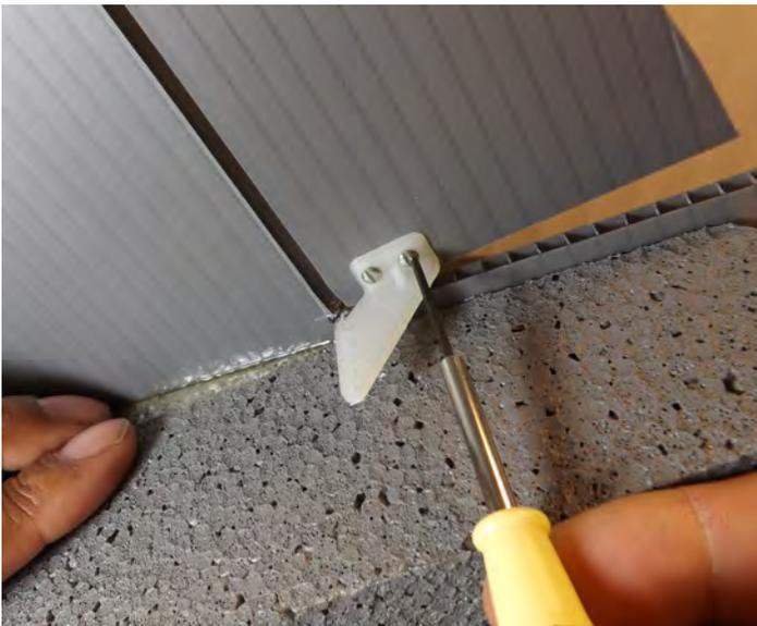
Attach the control horns to the elevons, don't over tighten.
