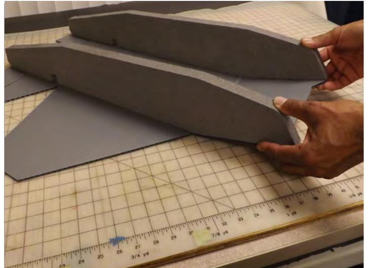
Press both nacelles to leading edge of the wing applying pressure on a smooth flat surface for 5 minutes until the epoxy cures
