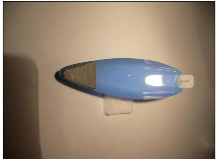
Epoxy the Coroplast® piece and glue canopy hinge into place to the inside of the canopy, after painting the outside of the canopy.
