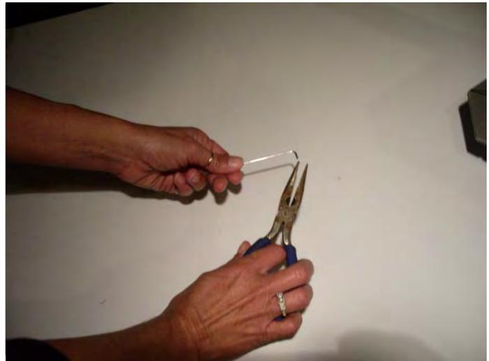
Bend the cut end to accommodate the push rod keeper.
