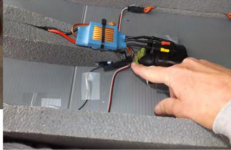
Embed electronic speed control battery wires in slot. Use double sided tape to hold speed control in place.
