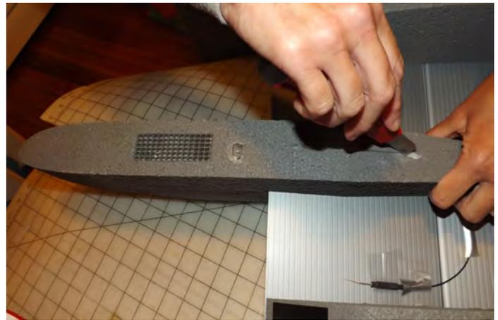
Cut slot for electronic speed control wires, it may be necessary to extend you electronic speed control battery wires in order to reach battery connector exit. Single knife cut is sufficient here, then use flat tip screw driver to open slot.
