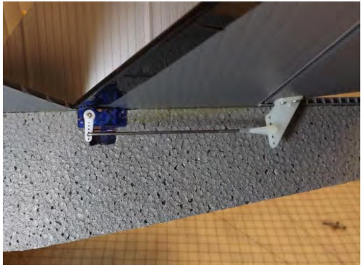
Connect the push rod to the servo arm 2<sup>nd</sup> hole from end and control horn middle hole. Repeat steps for left side.
