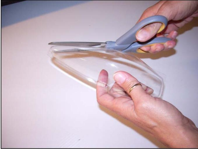
Carefully trim the canopy to fit the fuselage.
